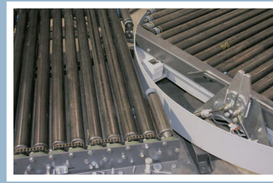
Contoured conveyors with smooth transfer
