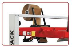
6-INCH TAPE HEAD (MOTOR OPTIONAL) Provides added security, preventing tampering, pilferage, and seals difficult to handle cartons.
