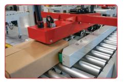
**"SOFT TOUCH" PNEUMATIC SYSTEM** Air powered belt drive and sealing section decreases product damage while maintaining presentation.
