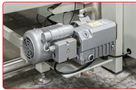
VACUUM PUMP SUCTION CUP SYSTEM Dedicated air system providing reliable erecting.
